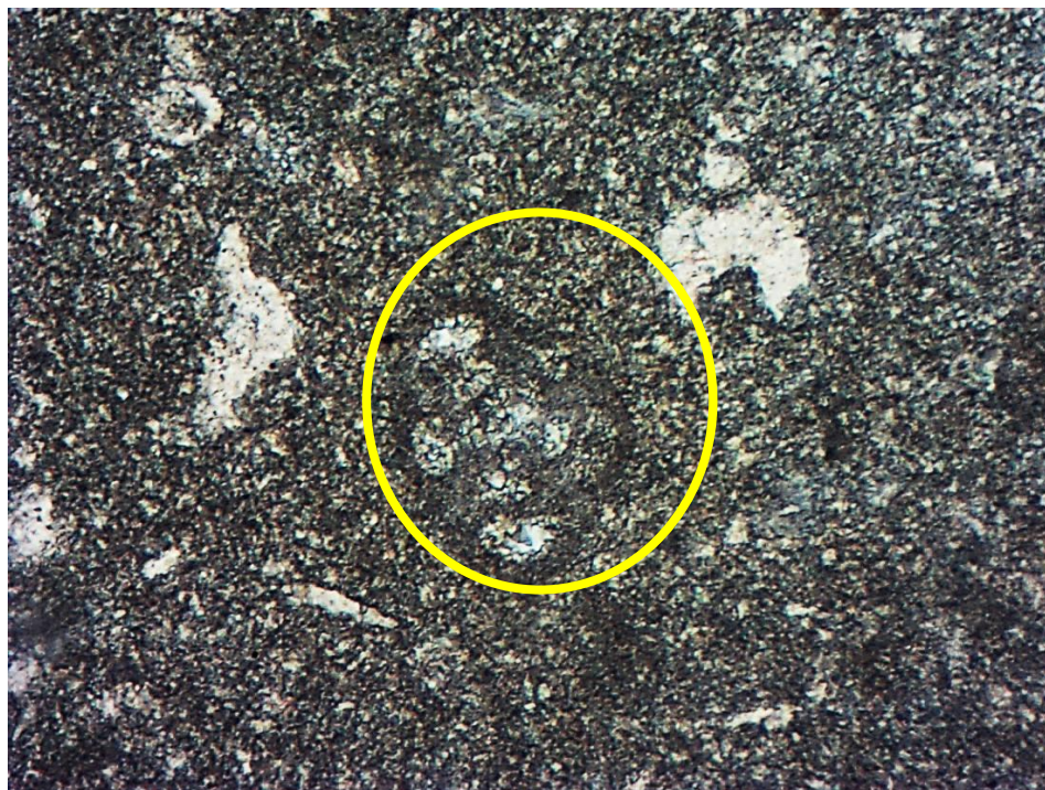
Fig. 9. Thin section photomicrograph showing microspar matrix formed due to aggrading neomorphic process of mudstone. Note: the foraminifera miliolid-test (yellow circle (10x-XPL).
