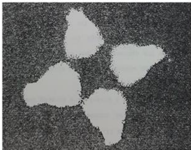
Fig. 2. Field emission pattern of a clean iridium tip surface.
