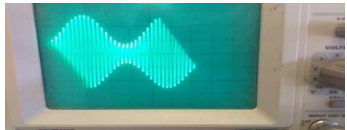
Fig. 32. The output amplitude modulated wave at point (b) after connecting the LC resonant circuit in Fig. 21 ( V_m = 6 V, V_c = 13 V).
