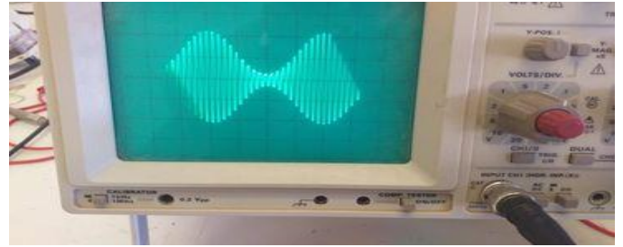
Fig. 29. The output amplitude modulated wave at point (b) after connecting the LC resonant circuit in Fig. 7. ( V_m = 6 V, V_c = 10 V).
